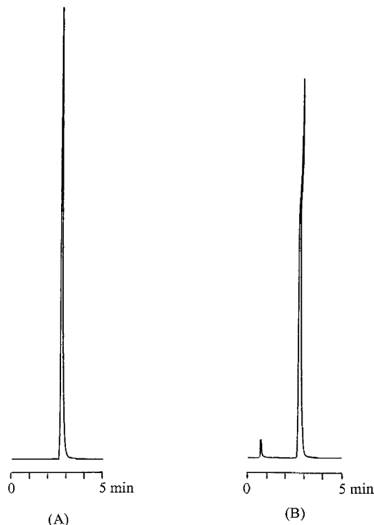
Fig. 1. Chromatograms at nominal conditions obtained on column B ( 75 \times 4.6 mm ID). (A) 0.10 mg/ml ketoconazole solution, and (B) 200 times diluted shampoo, t_R (ketoconazole) = 2.8 min.
